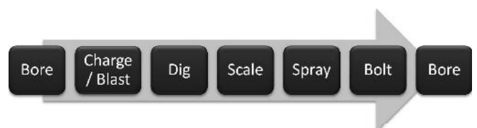
FIG 4 – Typical development mining cycle.
